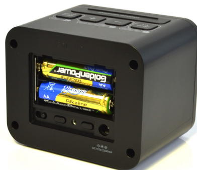
Rear View Showing back up batteries and DST, time set switches
